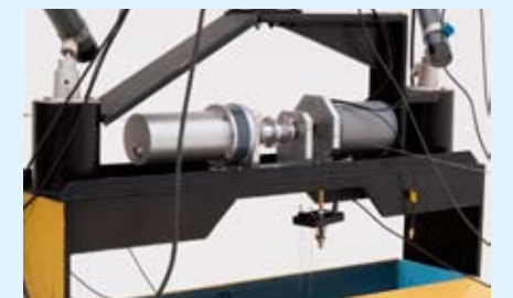
Schematic model of a hydraulic Power Take Off and actual PTO in a test modelling its hydraulic characteristics
